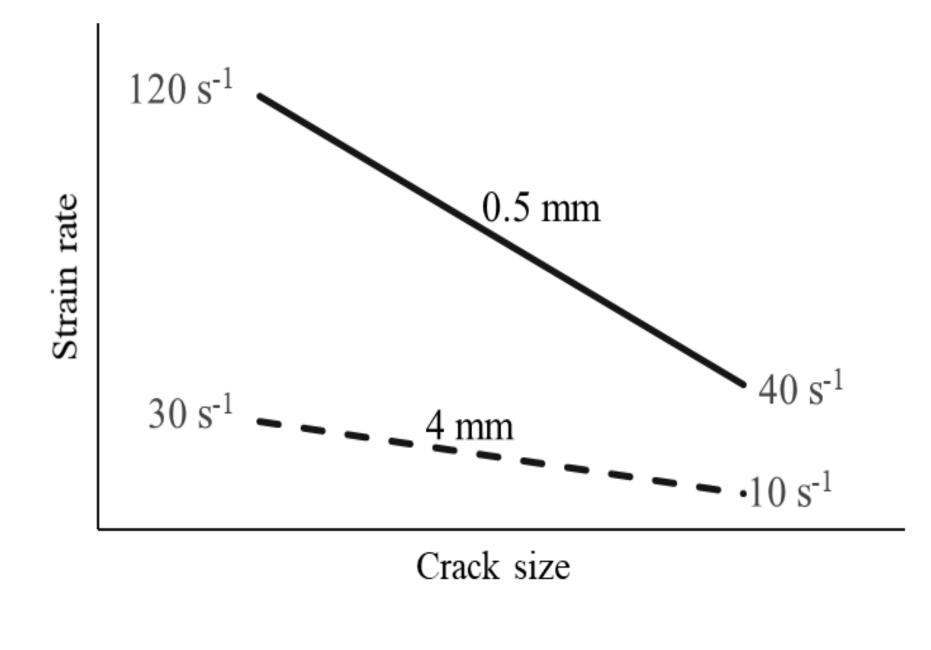
Figure 7 – True strain rate as a function of crack size for both adhesive thicknesses.
