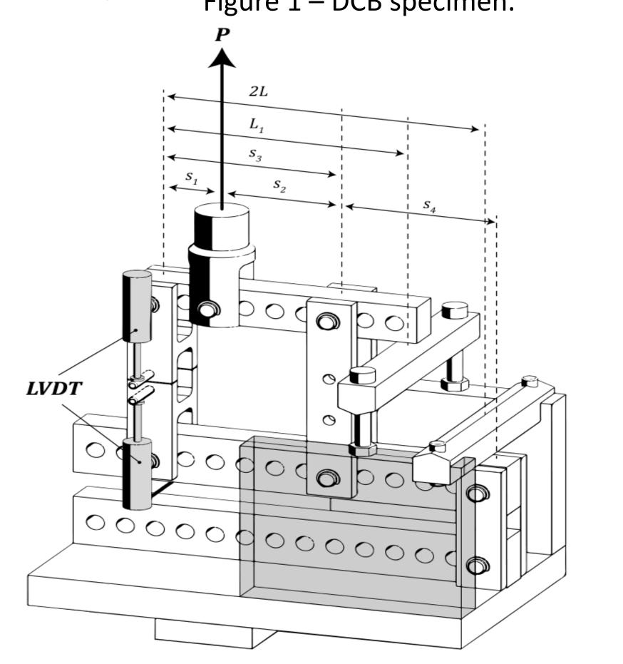
Figure 2 – Apparatus used for the mixed-mode loading conditions [1].
