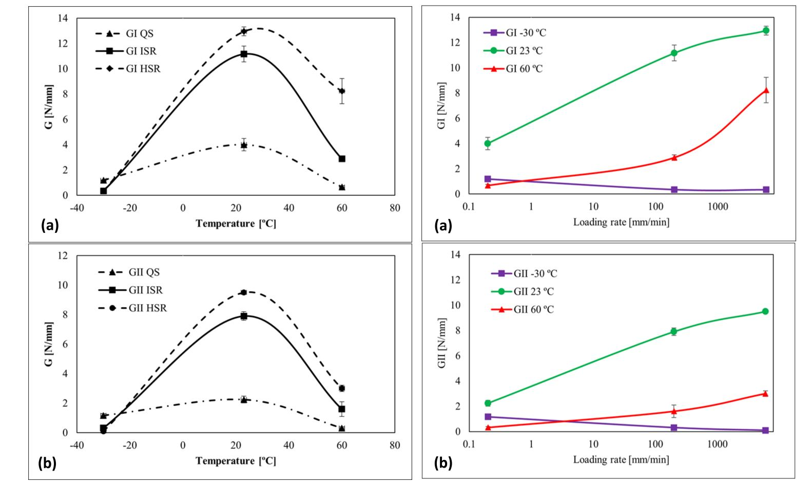
A ductile polyurethane-based adhesive with mechanical characteristics adapted for industrial purposes was employed throughout this study. The adhesive's glass transition temperature is -5 °C.
