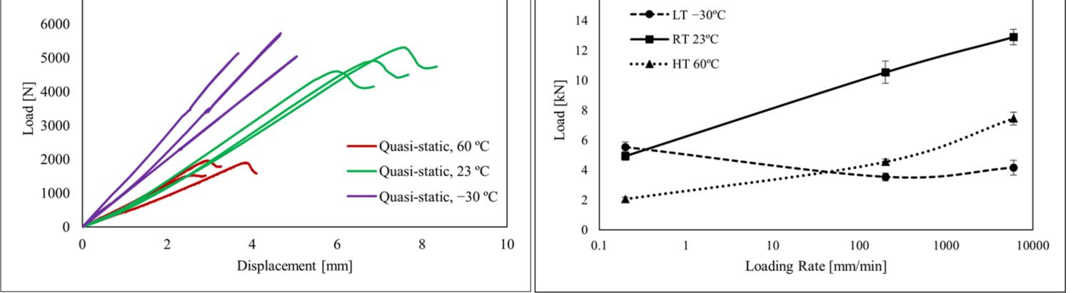
Figure 3 – Load-displacement of the machine for test submitted to quasistatic conditions for a mixed mode apparatus set up at 45°.
